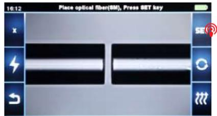
**Note:** If the splicer is set as "Auto mode", splicing will start automatically once the safety shield is closed.
