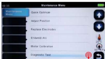
② Execute [Diagnostic test], then the following checks will be made.
