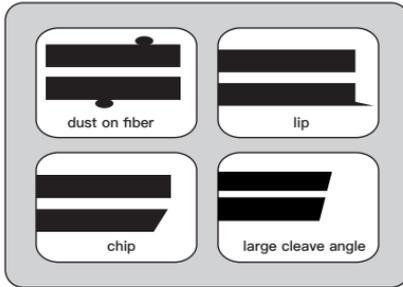
**Note:** The fibers are checked automatically when you press Splice button. The splicer automatically focuses the fibers and checks for damage or dust particles.
