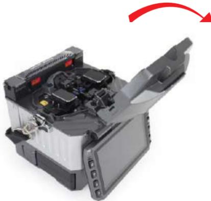
② Raise the fiber clamps. Position the fibers into V-grooves. Make sure the fiber ends are between the V-groove edges and the electrode tip.
