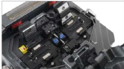
**Note:** Make sure to avoid sliding the fibers along V-grooves, but rather position them over V-grooves and tilt them down into place (as shown in the picture).
